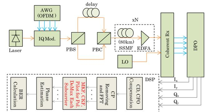
Fig. 4. Experimental setup of a polarization multiplexed CO-OFDM transmission. PB, polarization beam splitter; PBC, polarization beam combiner; SSMF, standard single-mode fiber; CD, chromatic dispersion; CFO, carrier frequency offset.
