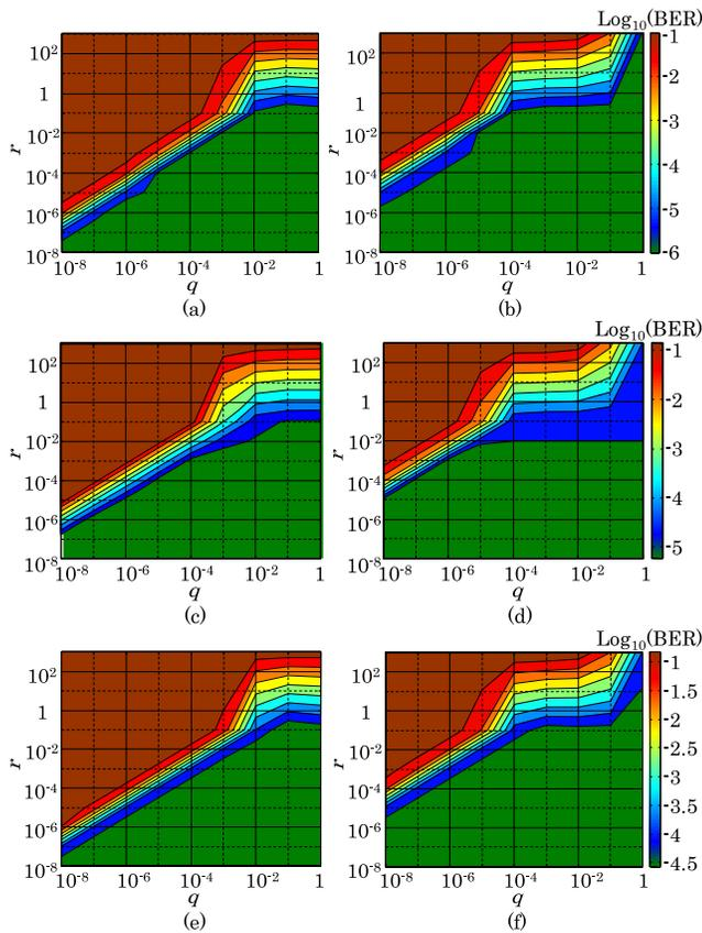
Fig. 5.  $q$ ,  $r$  versus  $\log_{10}$  (BER) with launch powers, fiber distances, and a Kalman filter being (a)  $-3$  dBm, 160 km, and CKF; (b)  $-3$  dBm, 160 km, and MKF; (c) 1 dBm, 160 km, and CKF; (d) 1 dBm, 160 km, and MKF; (e)  $-3$  dBm, 480 km, and CKF; (f)  $-3$  dBm, 480 km, and MKF.
