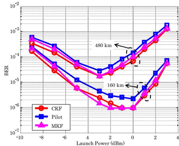
Fig. 6. BER versus launch power for three polarization de-multiplexing algorithms.
