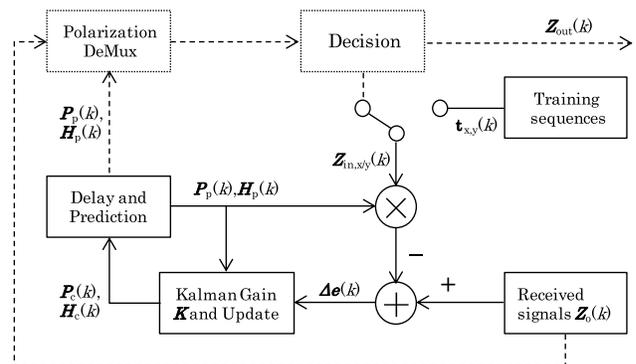
Fig. 1. Block diagram of the proposed polarization de-multiplexing with the MKF scheme.
