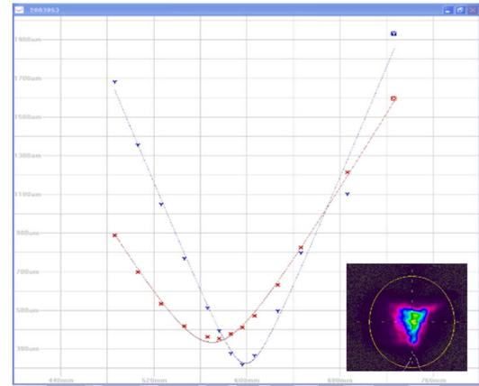
Fig. 6. Beam radius variation of the output laser.
