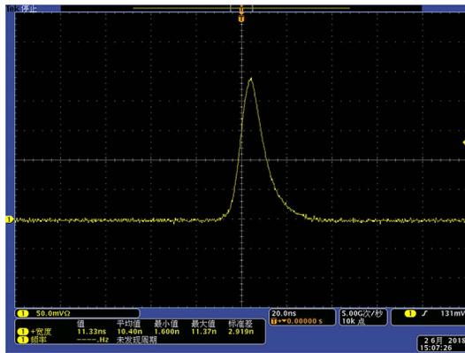
Fig. 4. Temporal trace of output laser pulse.
