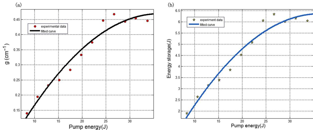
Fig. 2. (a) Small signal gain coefficient with different pump energy on single pass; (b) energy storage with different pump energy on single pass.
