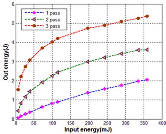
Fig. 3. Output pulse energy as a function of seed energy.
