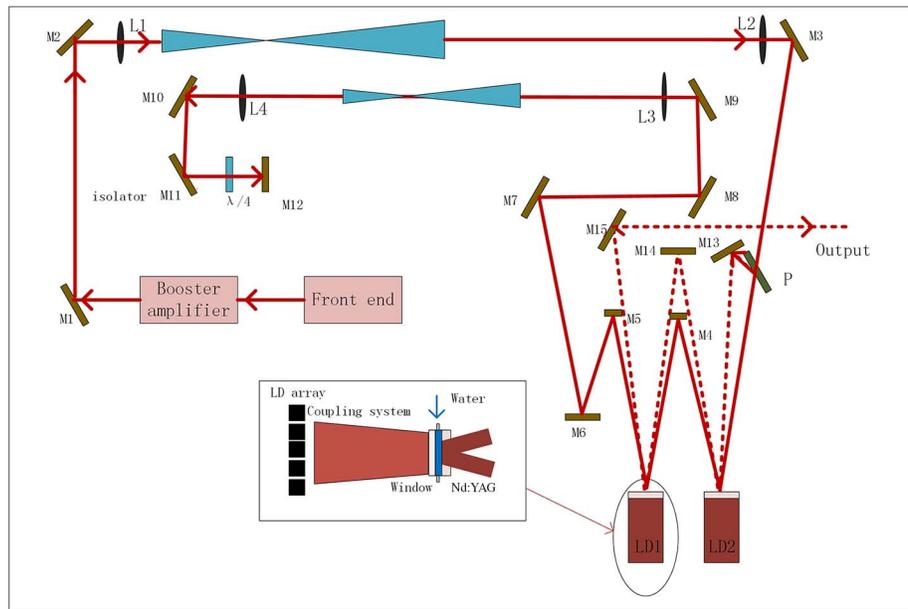
Fig. 1. Light path schematic of the laser amplifier system: M1–M15, high reflection (HR) at 1064 nm.
