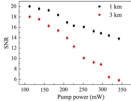
Fig. 5. SNR as the pump light power changes in two kinds of fiber length.
