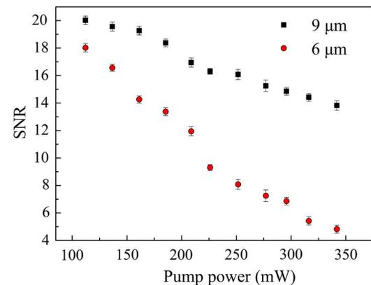
Fig. 3. SNR as the pump power changes in two kinds of fiber core diameter.
