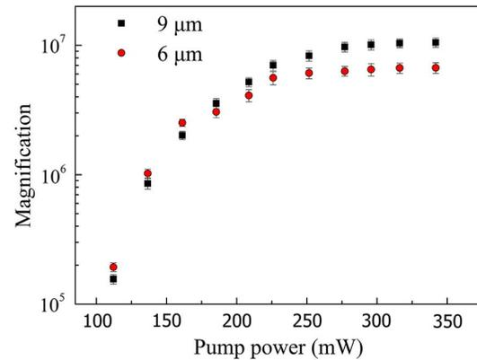
Fig. 2. Stokes peak power magnification as the pump power changes in two kinds of fiber core diameter.
