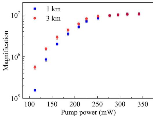
Fig. 4. Stokes peak power magnification as the pump light power changes in two kinds of fiber length.
