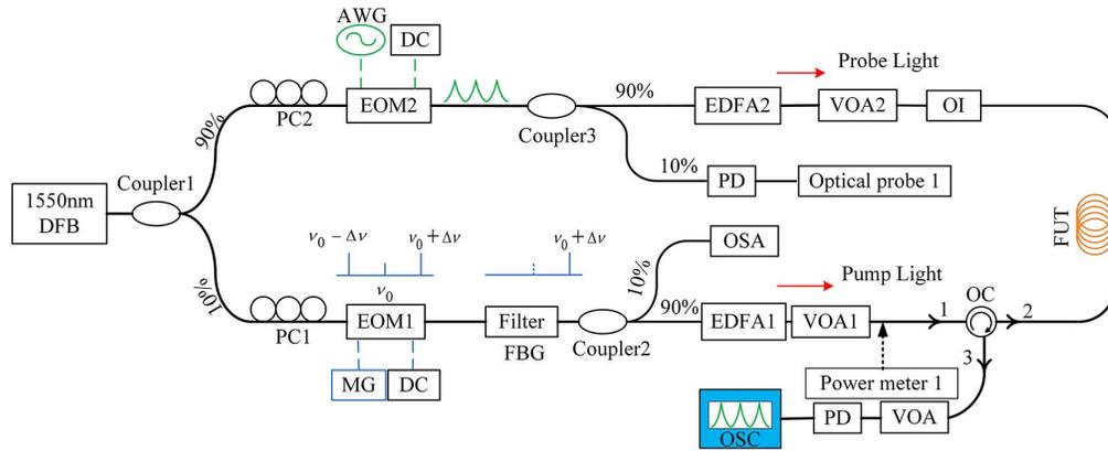
Fig. 1. Schematic diagram of the experimental setup. EOM, electro-optic modulator; EDFA, erbium-doped fiber amplifier; FUT, fiber under test; PC, polarization controller; AWG, arbitrary waveform generator; OI, optical isolator; PD, photodetector; MG, microwave generator; FBG, fiber Bragg grating; VOA, variable optical attenuator; OSC, oscilloscope; OC, circulator.
