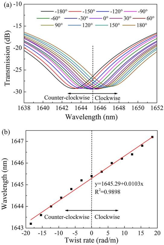
Fig. 4. (a) Transmission spectra and (b) wavelength shift of the NH-LPFG in response to the applied torsion in the non-polarization state.
