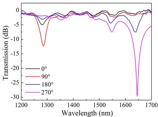
Fig. 2. Transmission spectra of the NH-LPFG under increasing rotation angles.
