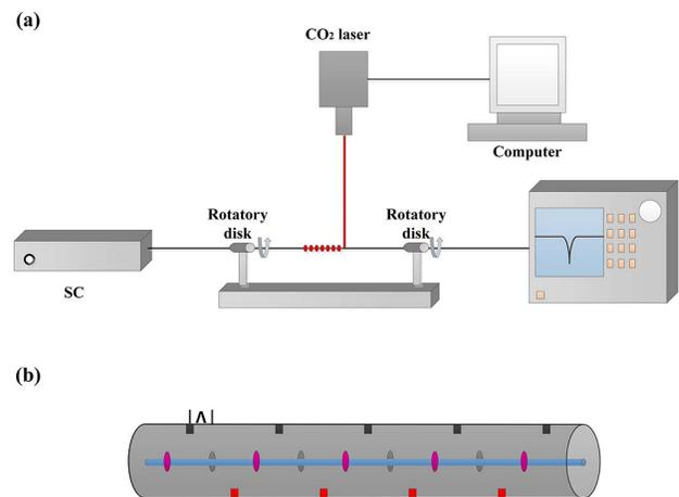
Fig. 1. (a) Experimental setup. (b) Schematic image of the NH-LPFG.
