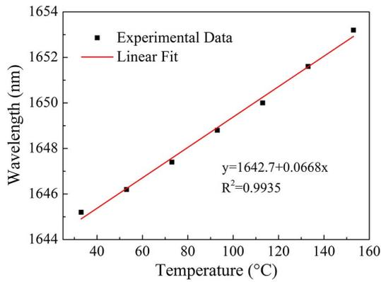
Fig. 7. Dependence of the resonance wavelength on temperature.
