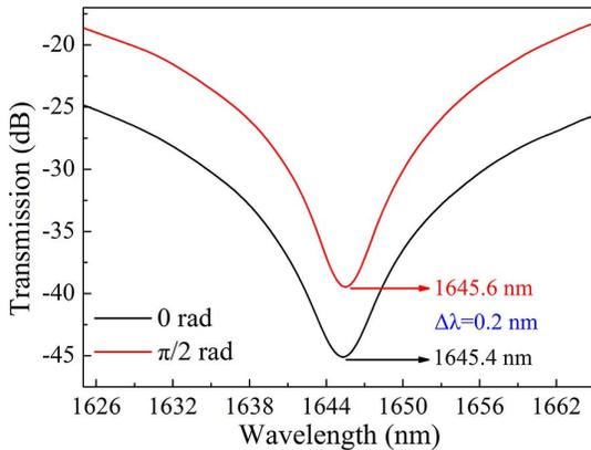
Fig. 5. Transmission spectra of the NH-LPFG in two polarization states.
