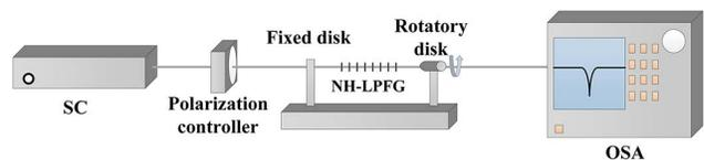
Fig. 3. Experimental setup for torsion measurement.
