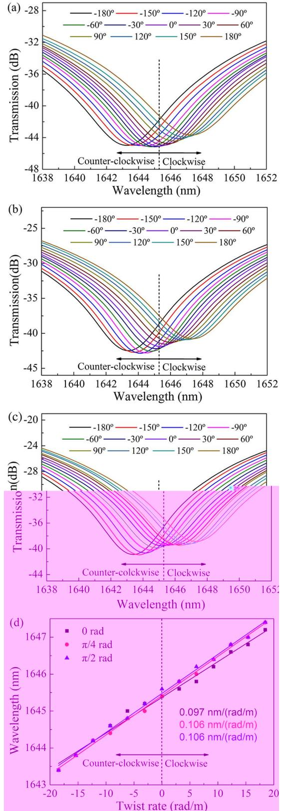
Fig. 6. Transmission spectra for the NH-LPFG in (a) 0 rad, (b)  $\pi/4$  rad, and (c)  $\pi/2$  rad polarization states under an applied torsion ranging from  $-18.3$  to  $18.3$  rad/m. (d) Wavelength shift of the NH-LPFG versus the different torsion angles in three polarization states.
