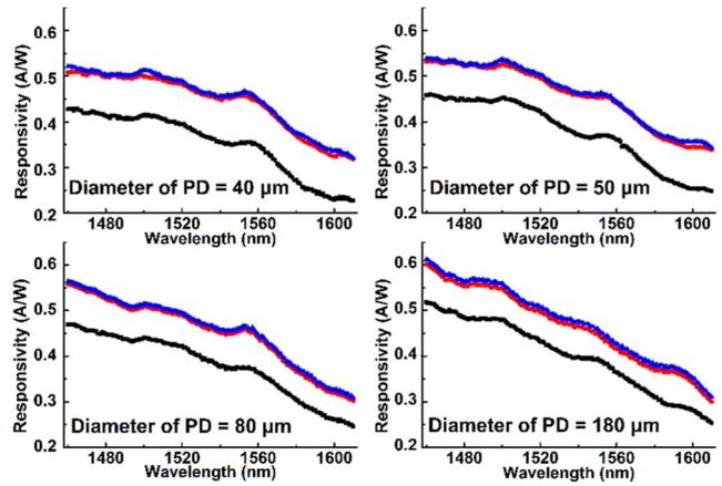
Fig. 5. Measured response spectra of different devices, when the reverse bias is  $3 \text{ V}$  and the input power is  $1.46 \text{ mW}$ . The black lines correspond to the original PD that is not integrated with a reflector. The red curves and the blue curves represent the PD integrated with S-SWGs and CC-SWGs, respectively.
