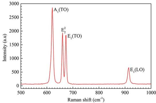
Fig. 4. Raman spectrum of the polished AlN under ambient conditions.
