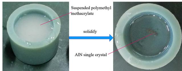
Fig. 1. Solidification process of the grinding sample.
