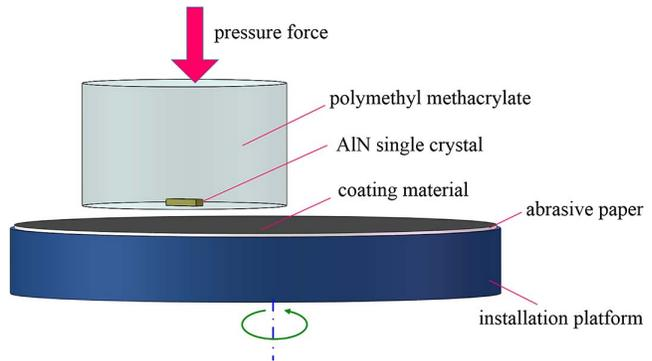
Fig. 2. Schematic illustration of the polishing process.
