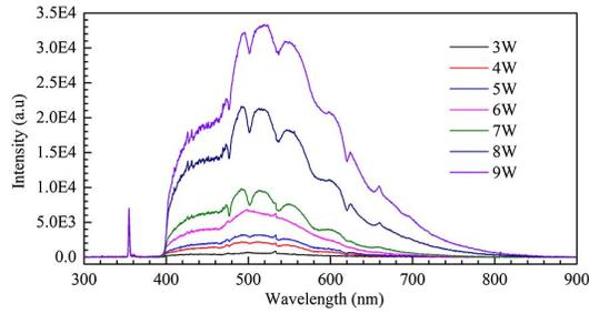
Fig. 6. Supercontinuum evolution with different pump powers at 355 nm.
