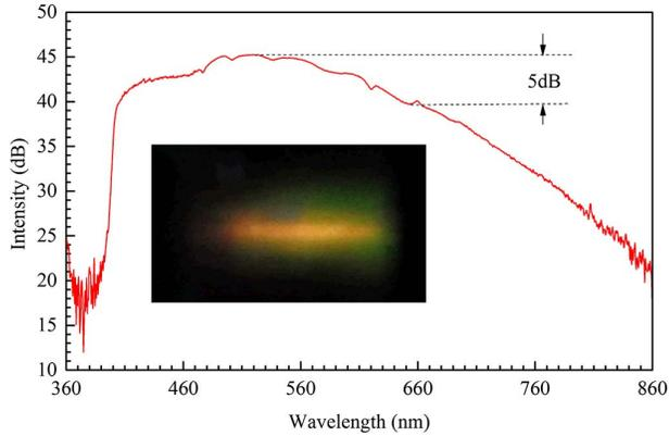
Fig. 7. Output spectrum at the maximum pump power of 9 W. Inset: the corresponding output far-field beam profile.
