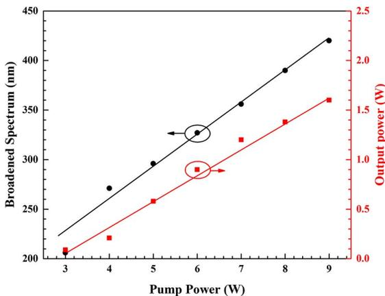
Fig. 8. Relationship between the output characteristics and the input pump power.
