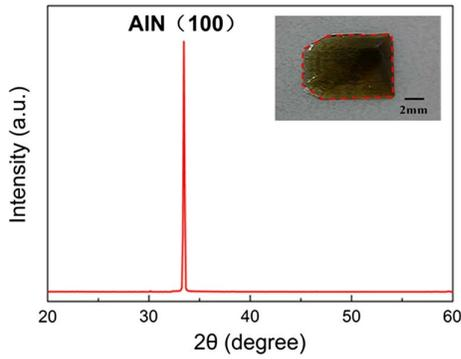
Fig. 3. XRD spectrum of the as-obtained AlN crystal. Inset: photograph of the polished AlN single crystal.
