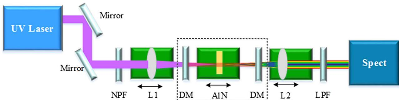
Fig. 5. Experimental setup for the SC generation. UV laser: 355 nm laser; Mirror: flat mirror with protected aluminum; NPF: narrow-bandpass filter; L1, L2: UV-fused silica plano-convex lenses; DM: dichroic mirrors HT@330–360 nm and HR@385–450 nm; LPF: longpass filter; Spect: spectrometer.
