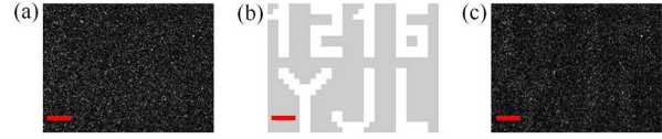
Fig. 6. (a) Speckle pattern of the illumination wave. (b) Object constructed using the DMD. (c) Intensity of the reflected wave of the object. Scale bar: 1000 \mu\text{m} .
