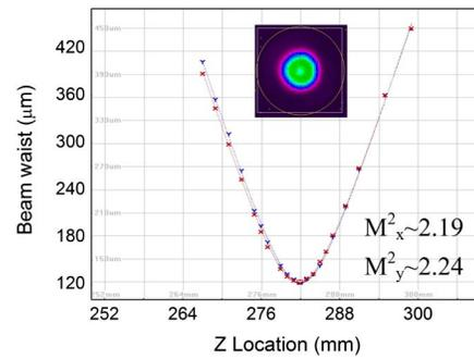
Fig. 4. Beam quality of the output laser.
