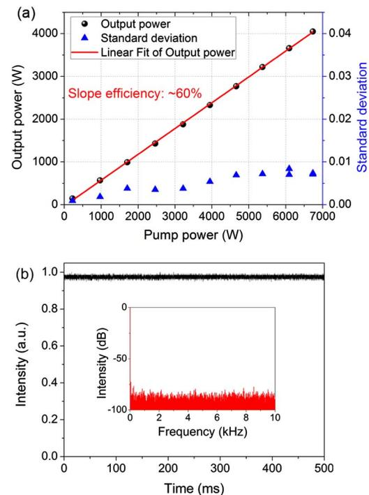
Fig. 2. (a) Output power and standard deviation of the temporal signals at different pump powers, (b) the temporal signal of the output laser and its Fourier spectrum at the operation of 4.05 kW.
