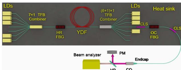
Fig. 1. Experimental setup (LDs, laser diodes; YDF, ytterbium-doped fiber; CLS, cladding light stripper; CO, collimator; PM, power meter; HR, high reflector).
