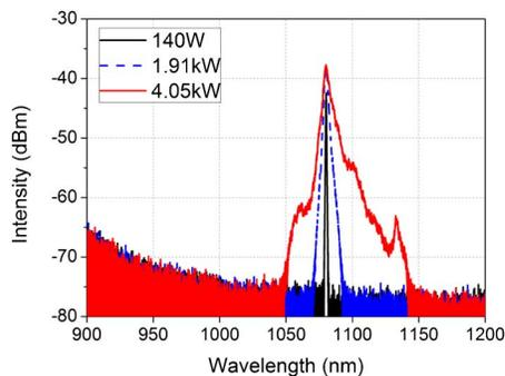
Fig. 3. Optical spectra of the output laser at different power levels.
