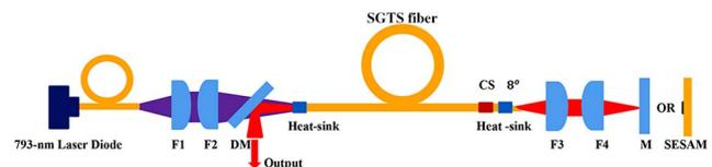
Fig. 3. Setup schematic of the laser experiments. DM: dichroic mirror; SGTS fiber: sol-gel fabricated Tm-doped silica fiber; CS: cladding stripper.
