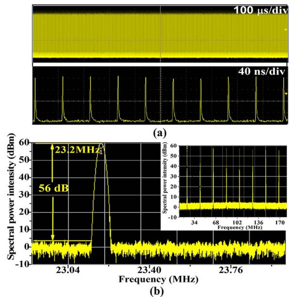
Fig. 5. (a) Mode-locked pulse trains in ms and ns time scales. (b) The radio frequency (RF) spectrum. Inset: the RF spectrum with a wide span.
