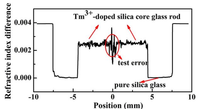
Fig. 2. Refractive index profile of the Tm-doped silica glass preform.
