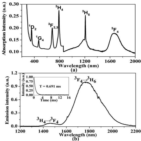
Fig. 1. Spectroscopic characteristics of LC SGTS fiber. (a) The absorption spectrum. (b) The fluorescence spectrum and fluorescence decay curve (inset) of the  ${}^3\text{F}_4 \rightarrow {}^3\text{H}_6$  transition.
