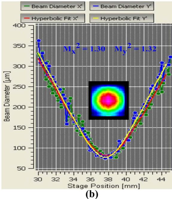
Fig. 4. (a) CW output power versus launched pump power. The inset shows the CW laser spectrum. (b) The  $M^2$  factors of the output laser beam. Inset: output laser beam profile.
