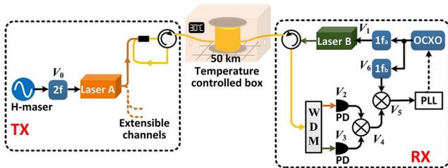
Fig. 4. Schematic diagram of non-harmonic precision reference frequency synchronization scheme.  $1f_a$ , 1 GHz + 130 Hz signal phase-locked to OCXO;  $1f_b$ , 1 GHz - 130 Hz signal phase-locked to OCXO.
