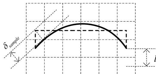
Fig. 4. Deviation induced by digitalizing the curve.
