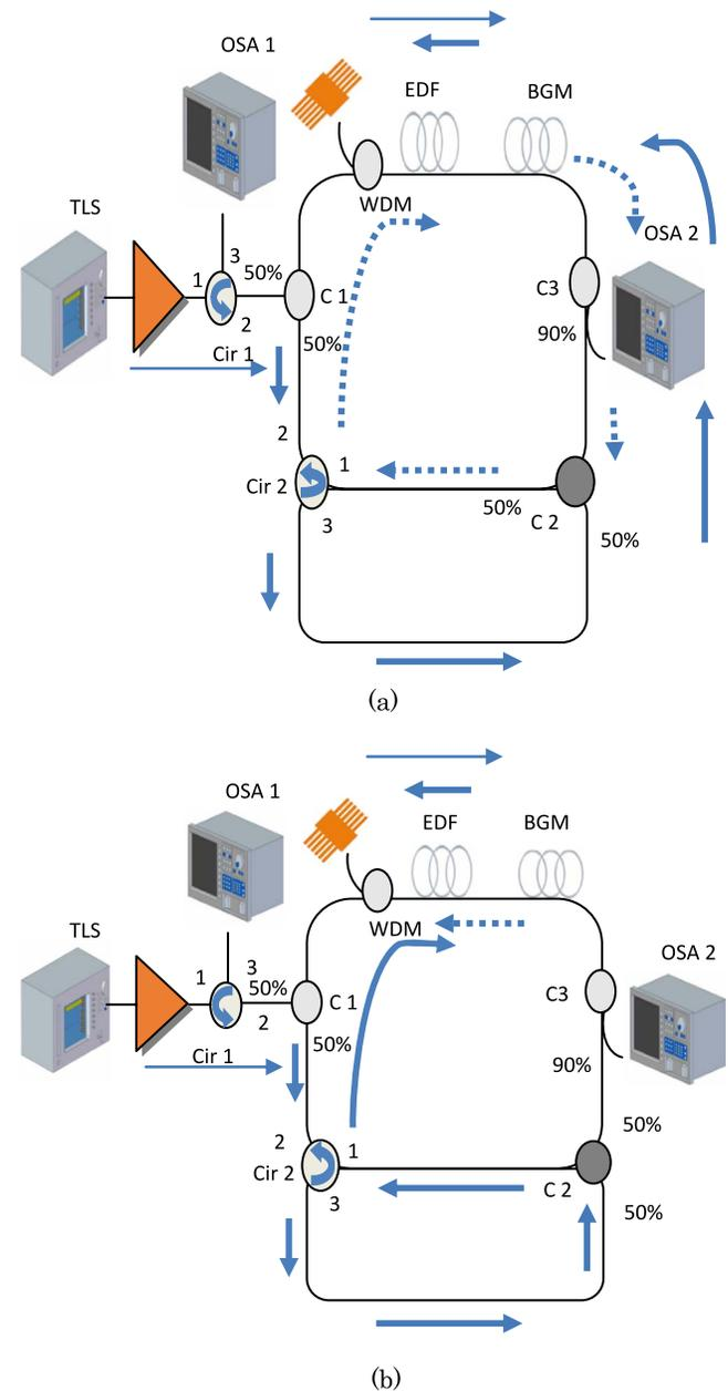
Fig. 1. Experimental setup of switchable spacing MWBFL. (a) Double Brillouin spacing: propagation of injected TLS (thin solid arrow), propagation of first BS (thick solid arrow), propagation of second BS (thick dashed arrow); (b) single Brillouin: propagation of injected TLS (thin solid arrow), propagation of first BS (thick solid arrow), propagation of second BS (thick dashed arrow).
