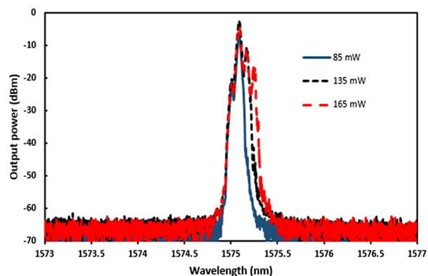
Fig. 4. (Color online) Output spectrum of SS-MWBFL at OSA 1.
