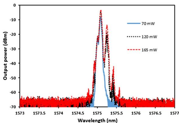
Fig. 2. (Color online) Output spectrum of DS-MWBFL (odd order) at OSA 1.
