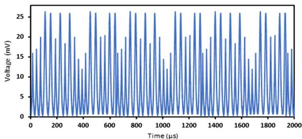
Fig. 5. Pulse train of Brillouin EDFL-based MWCNT SA.
