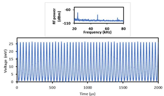
Fig. 7. Pulse train and RF spectrum of pulsed EDFL.
