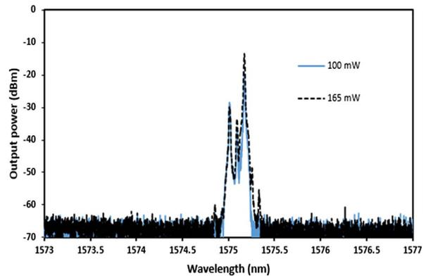
Fig. 3. (Color online) Output spectrum of DS-MWBFL (even order) at OSA 2.
