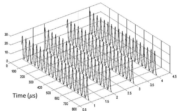
Fig. 8. Pulse train and RF spectrum of pulsed EDFL.
