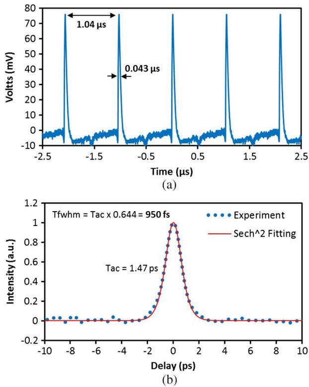
Fig. 6. (a) Oscilloscope train at a pump power of 165 mW. (b) The autocorrelation trace.
