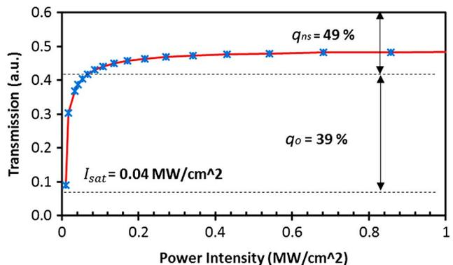
Fig. 3. Nonlinear optical absorption characteristics of the NiO-SA.
