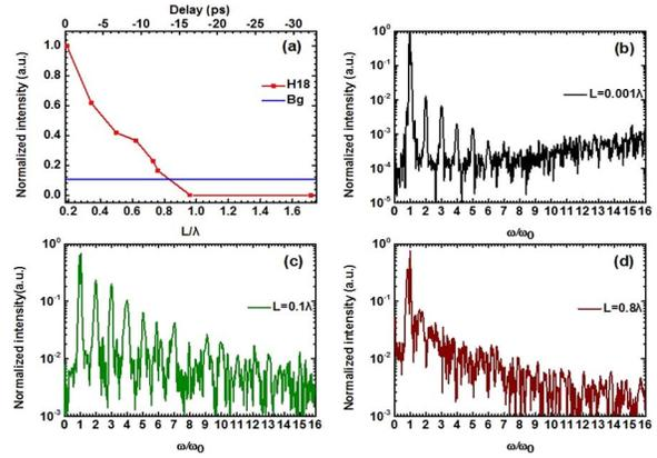
Fig. 4. (Color online) (a) Dependence of 18th harmonic intensities on the plasma scale lengths  $L$  obtained in the experiment (red). The blue line indicates the intensity of the background plasma emission. The harmonic spectra obtained by PIC simulations with different plasma scale lengths (b)  $L = 0.001\lambda$  (black), (c)  $L = 0.1\lambda$  (green), and (d)  $L = 0.8\lambda$  (brown).
