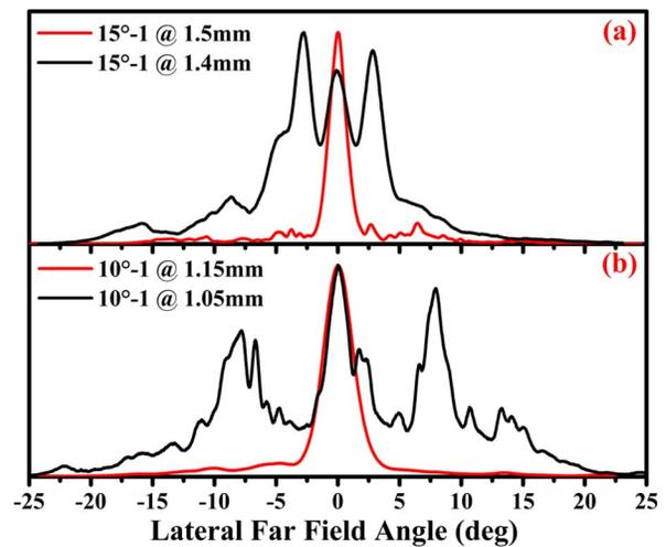
Fig. 5. (Color online) Lateral FF patterns of (a) VAC lasers with angle of  $15^\circ$  and cavity lengths of 1.5 and 1.4 mm, and (b) VAC lasers with angle of  $10^\circ$  and cavity lengths of 1.15 and 1.05 mm at 2.1  $\text{kA}/\text{cm}^2$ .
