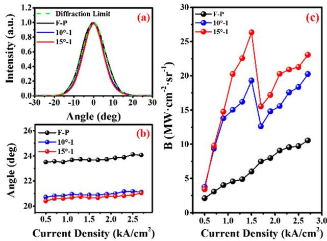
Fig. 9. (Color online) (a) Vertical FF profile of F-P and VAC lasers at  $2.7 \text{ kA/cm}^2$ , where the dashed line represents the diffractive limit, (b) vertical FF angles of F-P and VAC lasers as a function of current density, and (c) the brightness of VAC lasers and F-P lasers as a function of current density.
