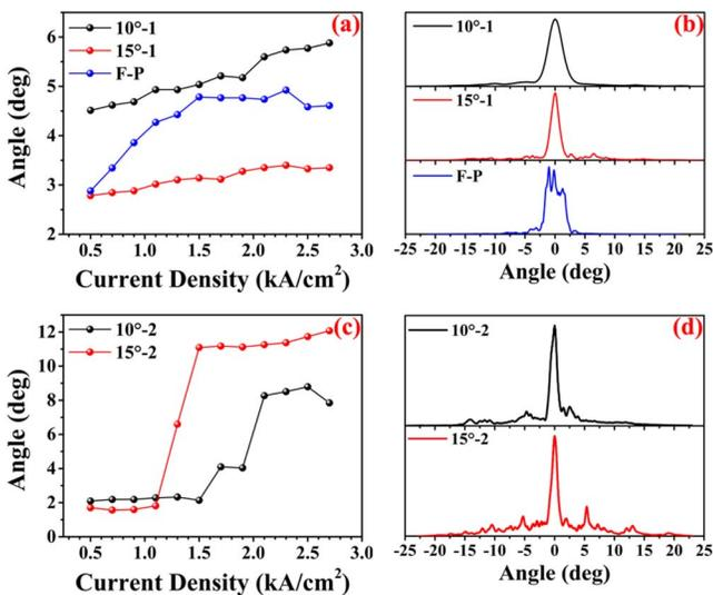
Fig. 4. (Color online) Lateral FF angles as a function of injected current density for emission from (a) facet 1 and (c) facet 2, (b) and (d) are the corresponding lateral profiles at 2.1  $\text{kA}/\text{cm}^2$ .
