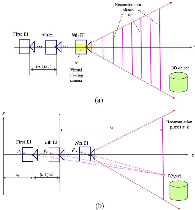
Fig. 2. Reconstruction process in ADS. (a) Multiple reconstruction planes. (b) Ray mapping between the reconstruction plane and elemental images.
