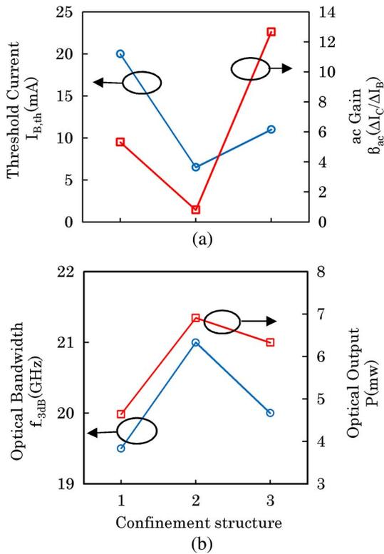
Fig. 6. Confinement structure dependency: (a) electrical and (b) optical characteristics of the SQW TL.
