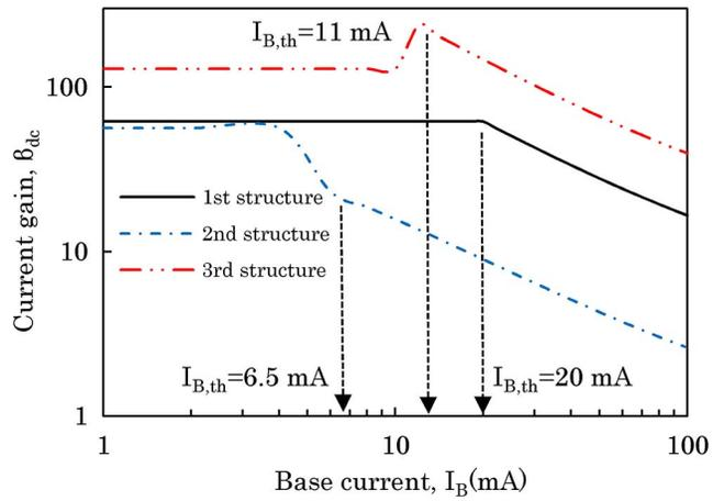
Fig. 3. Calculated dc gain  $\beta_{dc}(I_C/I_B)$ . The dc current gain reduces significantly, when the second structure is employed, because of the funnel form of this structure.
