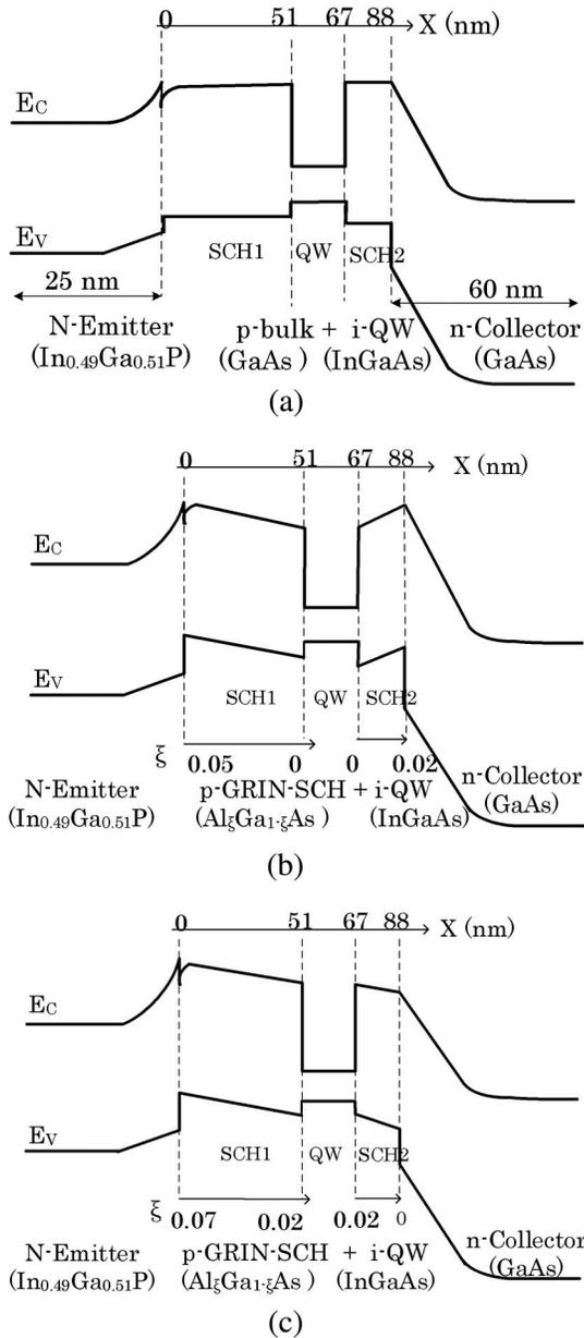
Fig. 1. Schematic energy band diagram of (a) the primary TL proposed by Feng and Holonyak<sup>[3]</sup> (first structure), (b) first proposed GRIN-SCH structure, (second structure), and (c) second proposed GRIN-SCH structure (third structure) under forward bias. Slope of the band diagram in SCH1 and SCH2, which determines the magnitude of the quasi-electric field.
