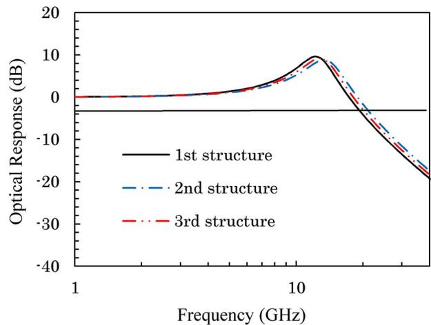
Fig. 5. Optical frequency response for the original and proposed GRIN-SCH structures. The  $-3$  dB bandwidth of the original TL (first structure) is  $\sim 19.5$  GHz, and for the second and third structures they are 21 and 20 GHz, respectively.
