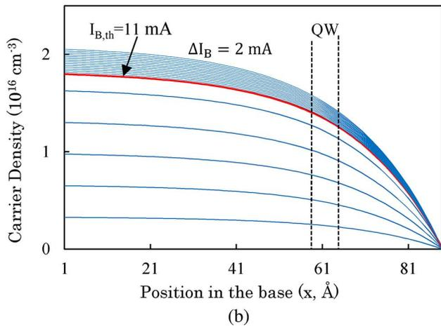
Fig. 2. Calculated minority electron distribution for (a) the first proposed GRIN-SCH structure and (b) the second proposed GRIN-SCH structure. (a) is in good agreement with the calculated carrier population for the GRIN-SCH QW laser<sup>[14]</sup>, and (b) also complies with the results of graded base HBTs<sup>[4]</sup>.
