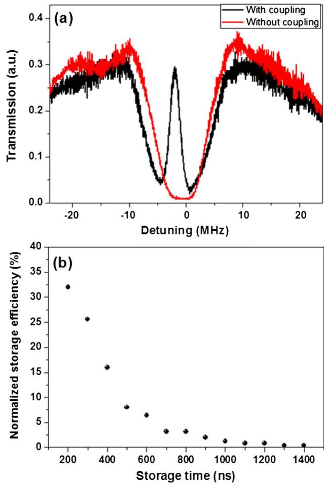
Fig. 2. (a) Transmission of the probe signal with (black) and without (red) coupling laser beam. (b) Storage efficiency as a function of storage time. The principal number of Rydberg excitation is 20.
