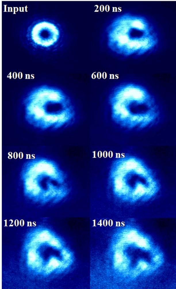
Fig. 3. Input and retrieval images of probe beam for various storage times at a principal quantum number of 20. Each image has the same dimensions and pixels. The central hole of the probe beam remains dark even for the longest storage time of 1400 ns.
