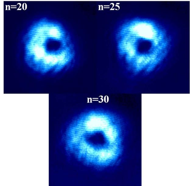
Fig. 4. Retrieval images of probe beam for various principal numbers of Rydberg excitation when the storage time is 300 ns.
