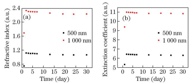
Fig. 4. (Color online) Variation of (a) refractive index and (b) extinction coefficient of Al films exposed in air at 500 and 1000 nm.
