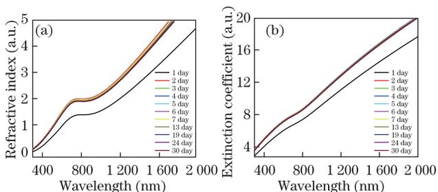
Fig. 3. (Color online) Variation of (a) refractive index and (b) extinction coefficient of Al films exposed in air for different days.
