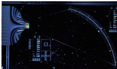
Fig. 6. Microscopic image of the fabricated EDG device.
