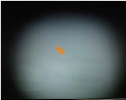
Fig. 2. Photograph of the displayed THz light beam spot at the focus point of the second OAP.
