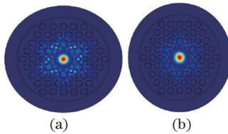
Fig. 1. Mode field distribution of Co-cage-PCF at  $90^\circ\text{C}$ : (a) at  $1064 \text{ nm}$ ; (b) at  $1550 \text{ nm}$ .
