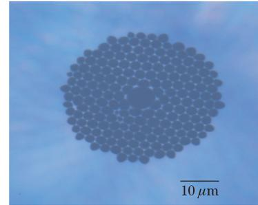
Fig. 4. Optical microscopic image of the end of HCPCF.
