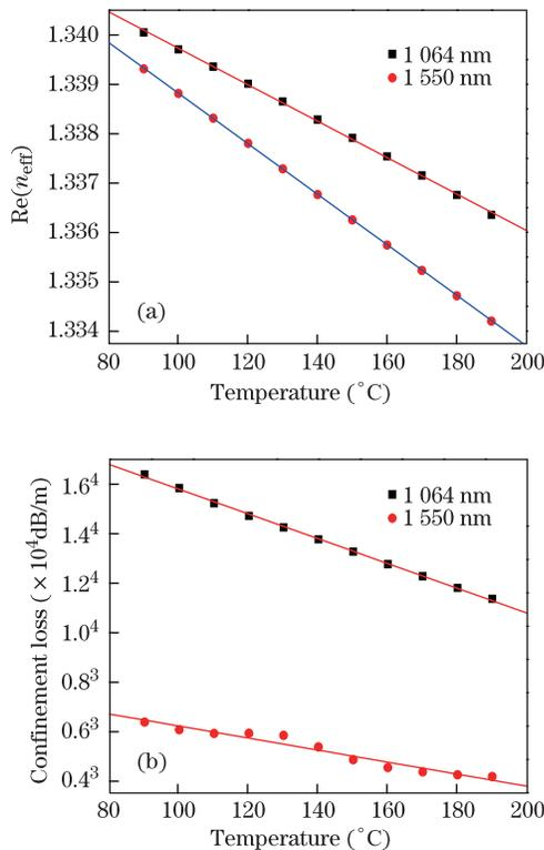
Fig. 2. (a) Dependence of the real part of mode effective refractive index of Co-cage-filled HCPCF on temperature and (b) the dependence of the confinement loss on temperature, which is related with the imaginary part of the effective refractive index.
