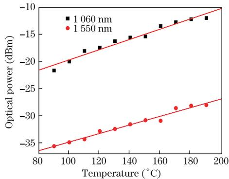
Fig. 6. Temperature dependence of transmission power for Co-cage-filled HCPCF at 1064 and 1550 nm.
