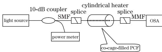
Fig. 5. Scheme of experimental setup for temperature sensor.
