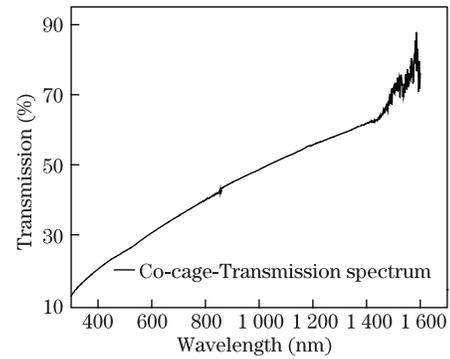
Fig. 3. Transmission spectrum of Co-cage from  $300$  to  $1600 \text{ nm}$ .
