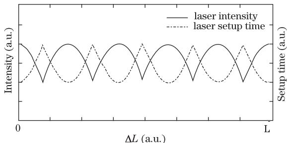
Fig. 1. Laser intensity and laser setup time versus cavity length relations.
