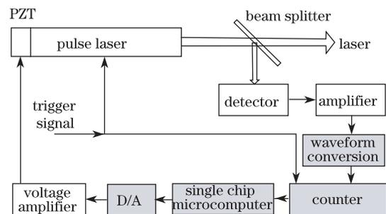
Fig. 2. Process of the frequency stabilization.
