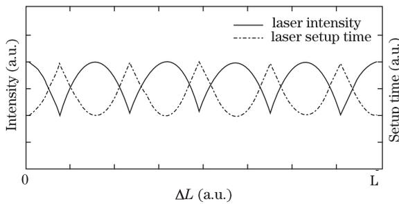
Fig. 1. Laser intensity and laser setup time versus cavity length relations.
