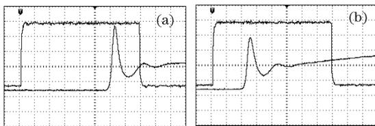
Fig. 4. (a) Trigger signal and laser waveform in the condition of open loop; (b) trigger signal and laser waveform in the condition of closed loop.
