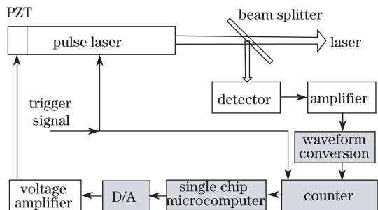
Fig. 2. Process of the frequency stabilization.
