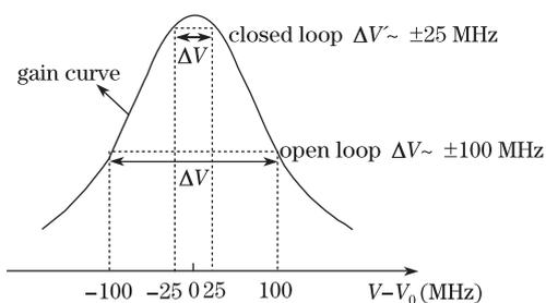
Fig. 6. Variances of the frequency under open- and closed-loop conditions.
