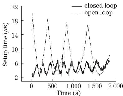
Fig. 5. Variances of the setup time in open- and closed-loop conditions.
