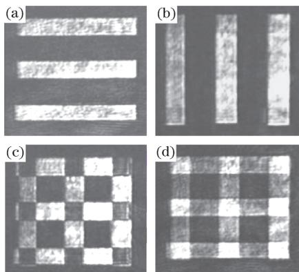
Fig. 4. Reconstruction image on CCD when polarizer  $P_3$  was set at different positions. The positions of polarizer  $P_3$  are  $90^\circ$  ( $270^\circ$ ),  $0^\circ$  ( $180^\circ$ ),  $26^\circ$  ( $206^\circ$ ), and  $154^\circ$  ( $-26^\circ$ ) to reconstruct the (a) parallel, (b) orthogonal linear holographies, (c) subtraction, and (d) summation image .
