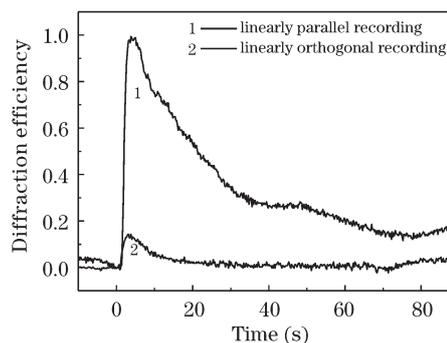
Fig. 3. Diffraction efficiency of the parallel and orthogonal linear polarization holographies.
