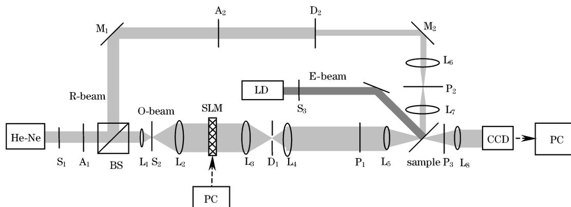
Fig. 2. Experimental setup of the polarization multiplexing holography.  $S_1 \sim S_3$ : shutter;  $A_1, A_2$ : attenuators; BS: polarizing beam splitters;  $L_1 \sim L_8$ : lenses;  $P_1 \sim P_3$ : polarizers;  $D_1, D_2$ : diaphragms;  $M_1 \sim M_3$ : mirror.
