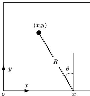
Fig. 2. Schema of scan conversion.
