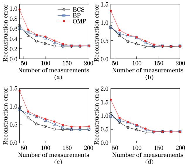
Fig. 4. Reconstruction errors for different CS algorithms. (a) Noiseless observation; (b) noisy observation with SNR=15 dB; (c) noisy observation with SNR=10 dB; (d) noisy observation with SNR=5 dB.
