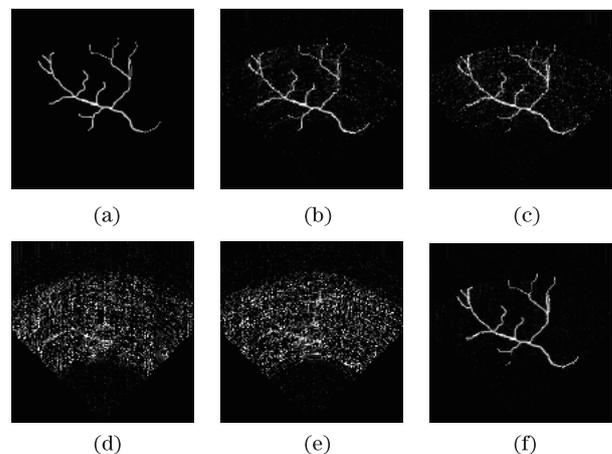
Fig. 3. Reconstruction of photoacoustic image from different CS methods using 100 masks. (a) Original image; (b) reconstruction from BP; (c) reconstruction from OMP; (d) reconstruction from STOMP-CFDR; (e) reconstruction from STOMP-CFAR; (f) reconstruction from BCS.
