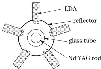
Fig. 3. Schematic of the laser head.
