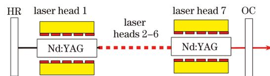
Fig. 1. Schematic diagram of the seven-rod resonator. HR: high-reflection mirror; OC: output-coupling mirror.
