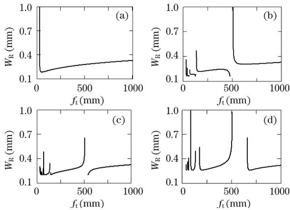
Fig. 2. Stable region of the seven-rod resonator. (a) The rod-rod distance  $d=100$  mm, the mirror-rod distance  $d_m=50$  mm; (b)  $d=100$  mm,  $d_m=60$  mm; (c)  $d=100$  mm,  $d_m=40$  mm; (d)  $d=100$  mm,  $d_m=100$  mm.
