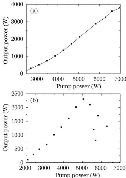
Fig. 4. Output power of the seven-rod resonator versus pump power. (a)  $d=100$  mm,  $d_m=50$  mm; (b)  $d=100$  mm,  $d_m=60$  mm.
