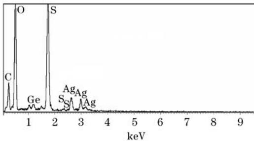
Fig. 2. EDXS of a probe after 150-s electroless silver plating.
