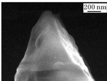
Fig. 4. SEM image of a probe apex area after 80-min electroless silver plating.
