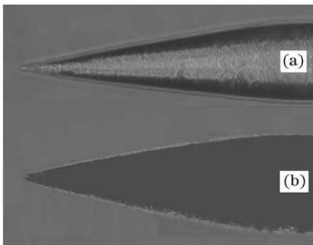
Fig. 3. Optical microscope images ( $\times 75$ ) of the probe (a) without plating and (b) after 80-min electroless silver plating.
