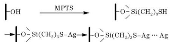
Fig. 1. Schematic illustration of electroless silver plating onto probe surface.
