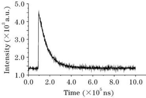
Fig. 3. Fluorescence lifetime of the Nd:KYW crystal.
