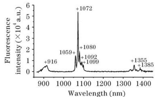
Fig. 2. Luminescence spectrum of Nd<sup>3+</sup>-doped KYW crystal at room temperature.
