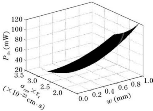
Fig. 4. Laser threshold  $P_{th}$  as function of the pump beam size  $w$  and the factor  $\sigma_{em} \times \tau_r$ .
