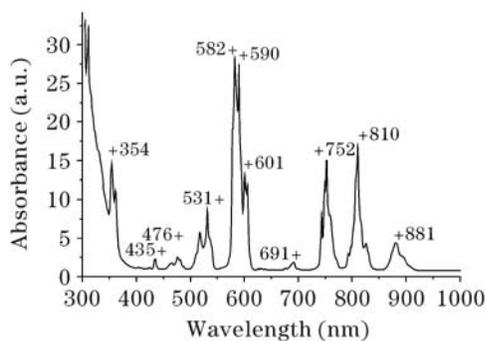
Fig. 1. Absorption spectrum of Nd<sup>3+</sup>:KYW crystal.
