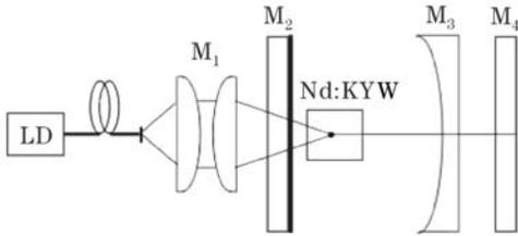
Fig. 5. Schematic of Nd:KYW laser resonator.
