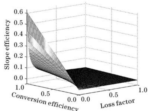
Fig. 7. Relationship among the slope efficiency, the conversion efficiency, and the loss factor.
