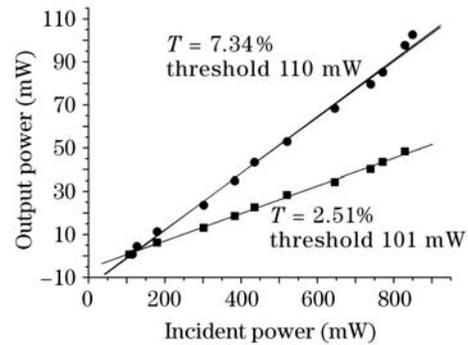
Fig. 6. Laser output power of Nd:KYW crystal at 1072 nm versus LD pumping power in the free-running mode.
