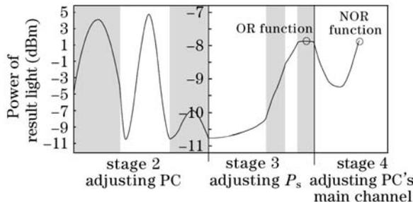
Fig. 2. Principle adjusting curve during stages 2–4.
