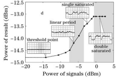
Fig. 3. Sample curve of  $P_r$  versus  $P_s$  and waveforms of result light at key points in stage 3.
