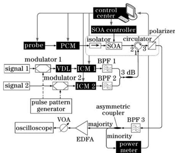
Fig. 1. Experiment setup of CPM OR/NOR AOLG. EDFA: erbium-doped fiber amplifier; VOA: variable optical attenuator; BPF: band-pass filter; VDL: variable delay line; ICM: intensity control module.
