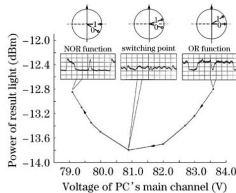
Fig. 4. Sample curve of  $P_r$  versus voltage of PC's main channel  $V_{main,PC}$  and waveforms of result light at key points in stage 4.
