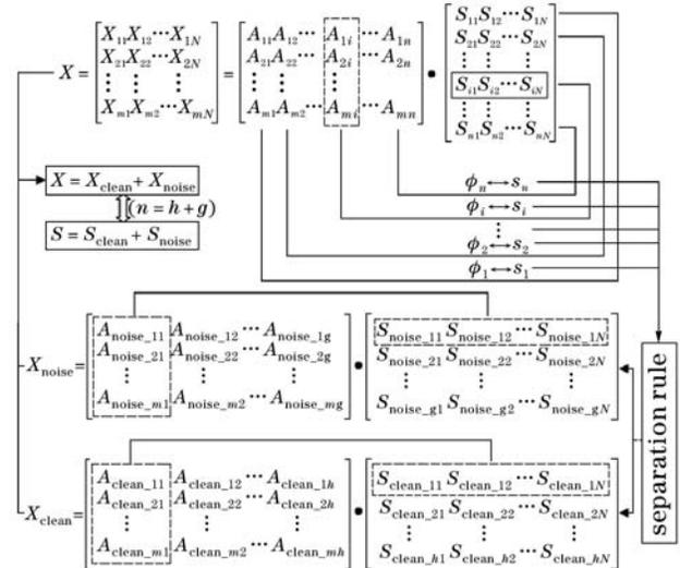
Fig. 1. Proposed principle for separation of basis images.
